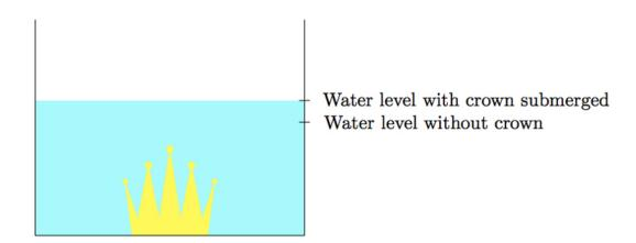
Measuring the two water levels indicated and subtracting gives the volume of the crown which is the same as the volume of the water displaced when it is submerged.
